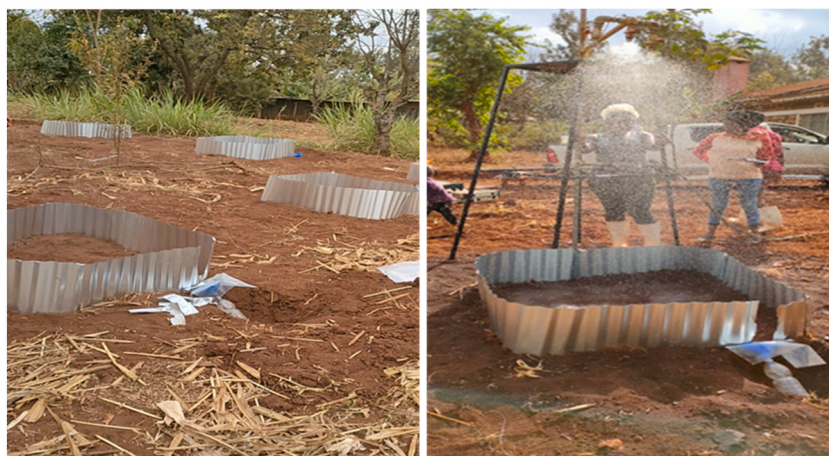
Fig. 3. A partial view of the experimental set up displaying the plot layout (left) and the rainfall simulation (right) in Meru-South Sub County in Tharaka-Nithi County.
