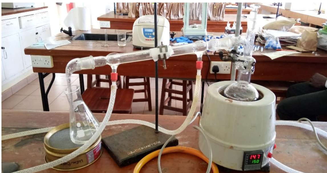
Plate 4: Sample distillation setup
