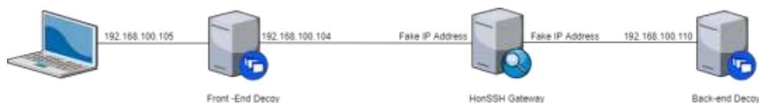
Figure 3.3: Integration of the front-end and back-end decoys
