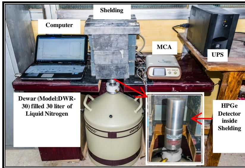
Figure 1. Represent all parts of HPGe system.
