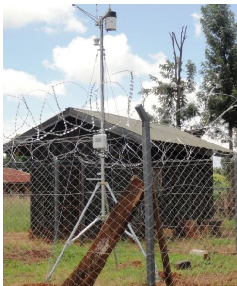
Plate 3. 2: Automatic rain gauge installed at the site
