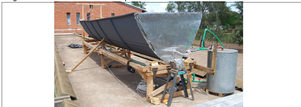
Figure 1: Fabricated prototype parabolic trough solar concentrator for steam production
