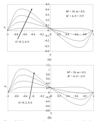
Figure 5. Primary  $(u_1)$  and secondary velocity  $(w_1)$  distribution for various values of G.
