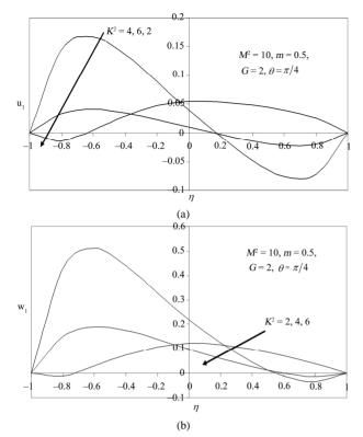
Figure 4. Primary  $(u_1)$  and secondary velocity  $(w_1)$  distribution for various values of  $K^2$  with  $\theta = \pi/4$ .
