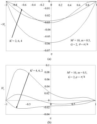
Figure 9. Primary  $(H_x)$  and secondary  $(H_z)$  induced magnetic field distribution for various values of  $K^2$  with  $\theta = \pi/4$ .
