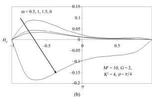
Figure 11. Primary  $(H_x)$  and secondary  $(H_z)$  induced magnetic field distribution for various values of *m*.
