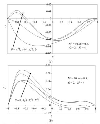
Figure 7. Primary  $(H_x)$  and secondary  $(H_z)$  induced magnetic field distribution for various values of  $\theta$ .
