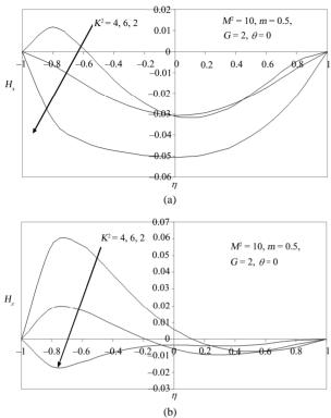
Figure 8. Primary  $(H_x)$  and secondary  $(H_z)$  induced magnetic field distribution for various values of  $K^2$  with  $\theta = 0$ .
