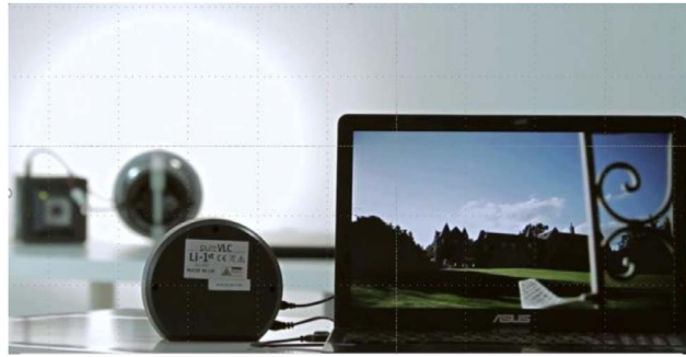
Fig. 7. This illustration shows the operation of a LiFi link under strict non-line-of-sight (LoS) conditions (courtesy pureLiFi).
