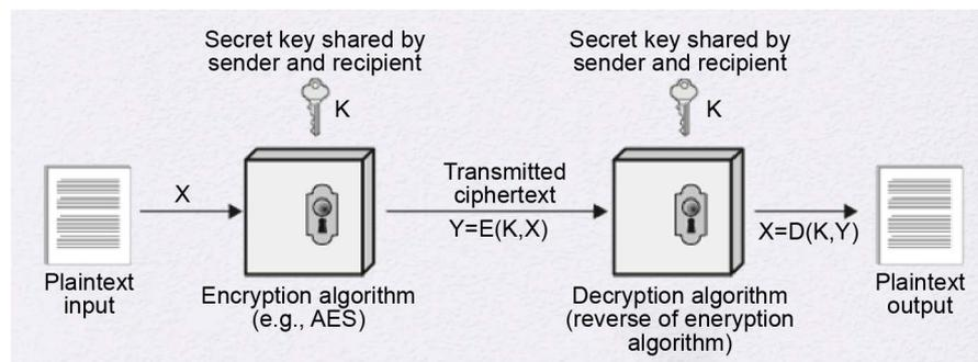
Figure 14. Cryptography symmetric encryption [3].
