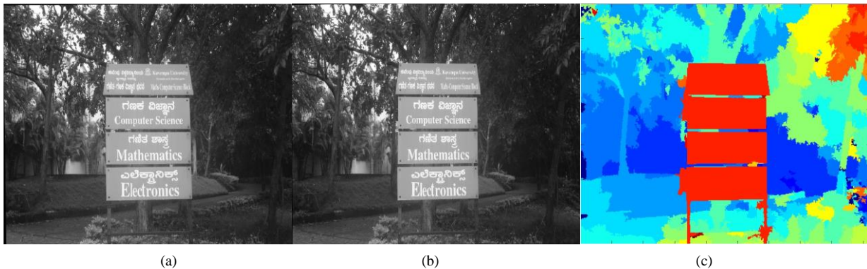
Fig.2. Results of Estimated Disparity Map: (a) Rectified Left Frame, (b) Rectified Right Frame and (c) Estimated Disparity Map.
