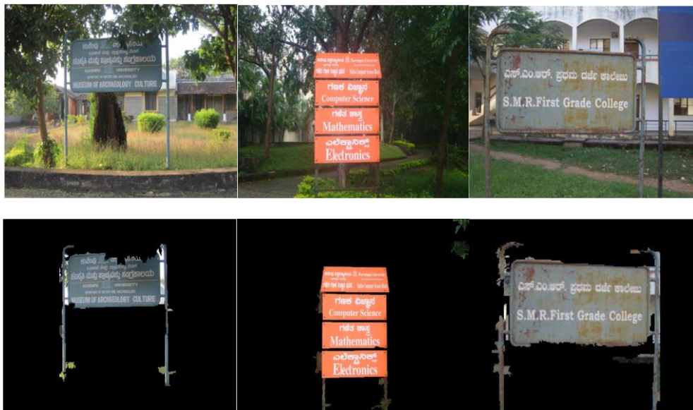
Fig.8. The Results of Planar Surface Extraction Obtained by Our Method on Video Frames of Our Dataset: First Row-Original Left Frames and Second Row-Extracted Planar Surface.
