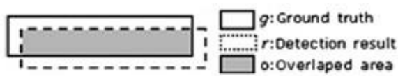
Fig.7. Illustration of the Overlap of A Ground Truth Box and Detected Bounding Box (Courtesy of Ye et al., 2005)
