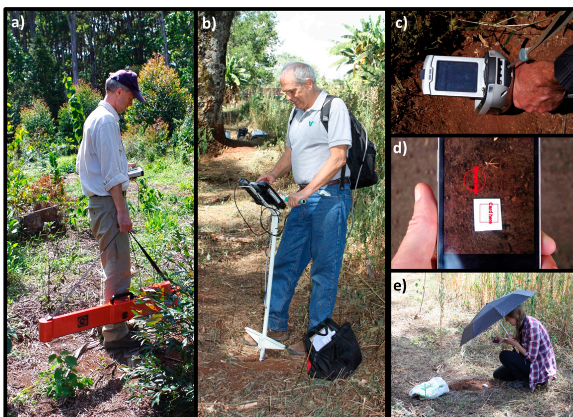
Figure 2. The proximal sensors tested: (a) an electromagnetic induction sensor; (b) an optical sensor; (c) a portable X-ray fluorescence sensor (PXRF); (d) a smartphone soil color application; and (e) the umbrella used for shading.
