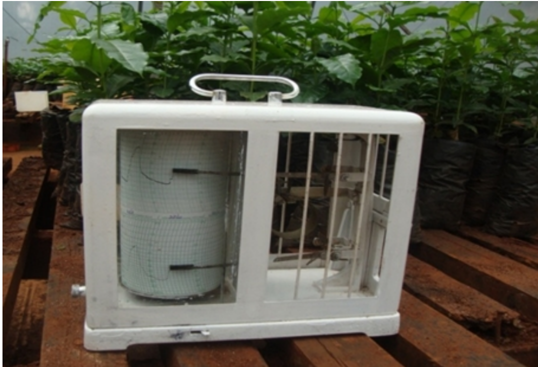
Plate 1. Thermo-hygrograph used to record temperatures and RH
