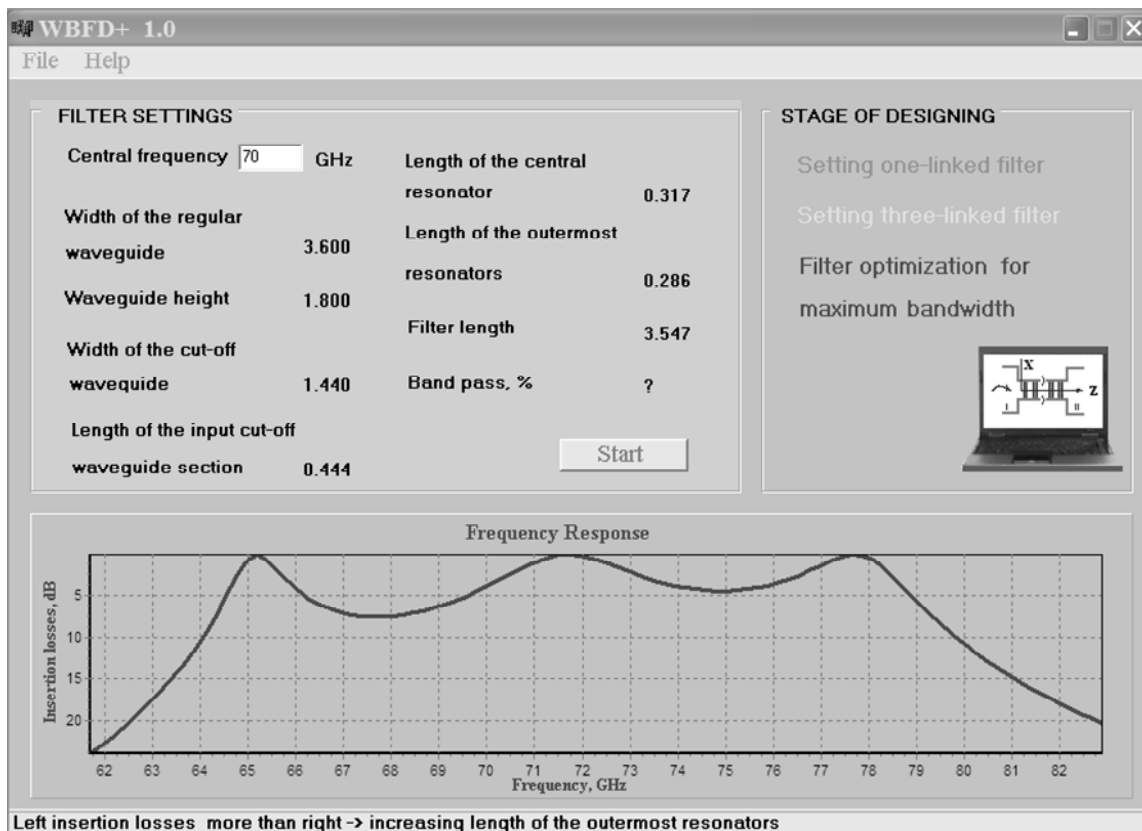
Figure 4. The intellectual CAD results at regime of FR3 module for three-tier filter.
